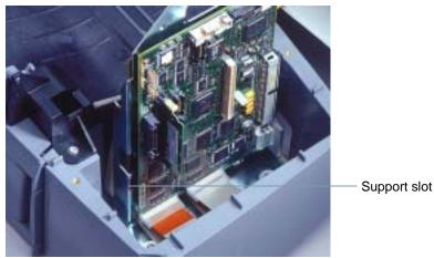
5. Press the imprinter board firmly into the main control board.
